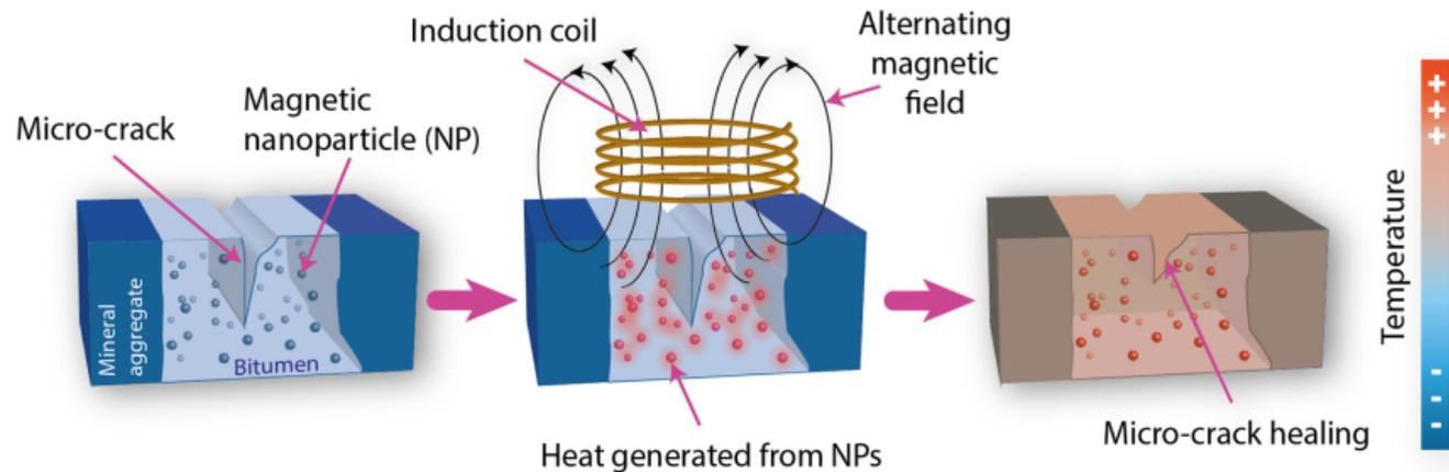
1. **Magnetic field** generated by **electrical current** in the coil
