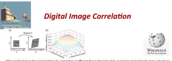
DIC is predicated on the maximization of a correlation coefficient that is determined by examining pixel intensity array subsets on two or more corresponding images and extracting the deformation mapping function that relates the images (Figure 1). An iterative approach is used to minimize the 2D correlation coefficient by using nonlinear optimization techniques. The cross correlation coefficient rij is defined as
